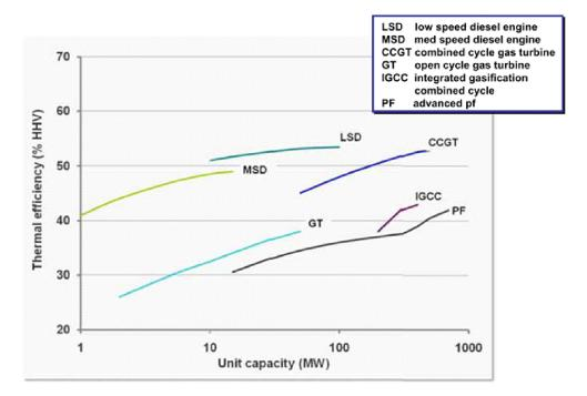
Figure 2-2 CSIRO thermal efficiency for electricity generation<sup>8</sup>
