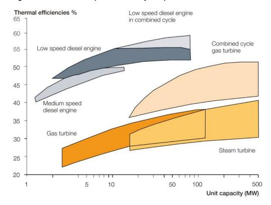
Figure 2-1 MAN Diesel power efficiency comparison at ISO 3046<sup>7</sup>
