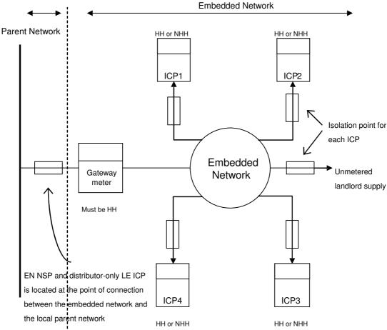
45. Note that an ICP identifier must also be assigned to the point of connection to the parent network (embedded network NSP). This is a distributor-only ICP with
