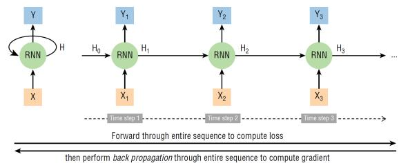
Figure 2: Back propagation process in RNNs to compute gradient values.
