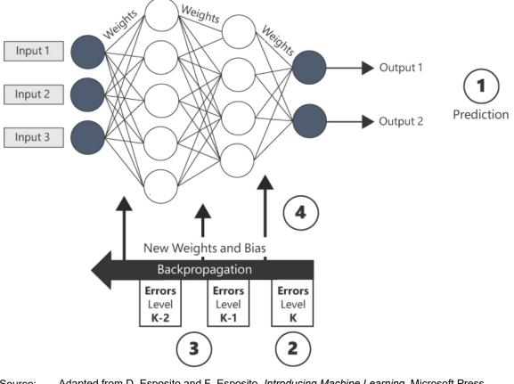
Figure 1: Simplest model is the feed-forward neural network with backpropagation algorithm. The network can have any number of nodes and layers.
