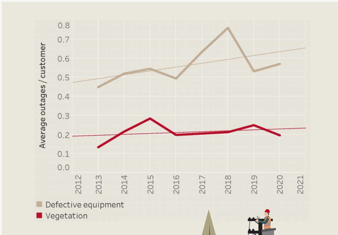
Figure 31: Average outages experienced by customers that were caused by defective equipment and vegetation
