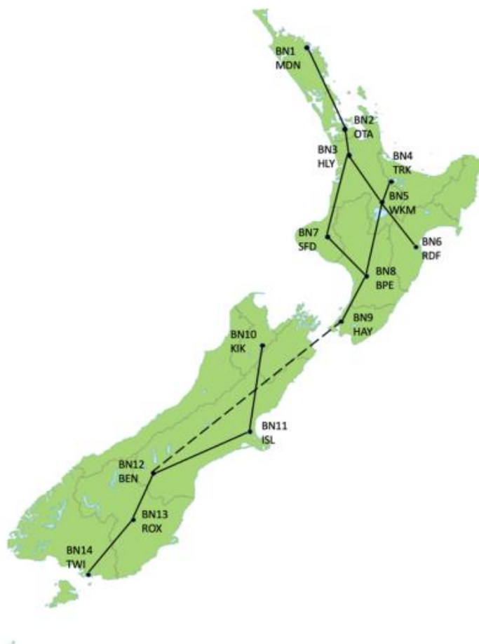
Figure 18 Simplified transmission grid with 14 backbone nodes
