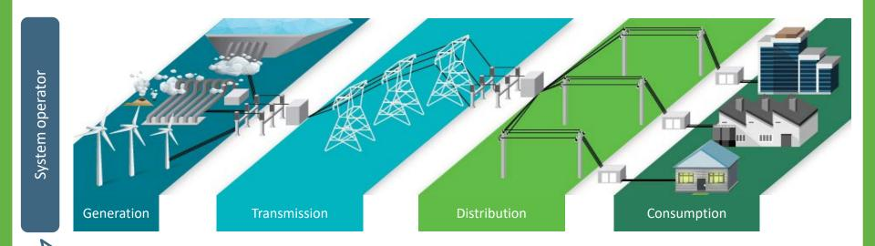
The system operator manages the power system so there is a continuous balance between electricity supply and demand.
