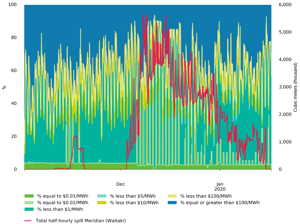
Figure 26: Waitaki Hydro Scheme Offer Bands and Flood Spill
