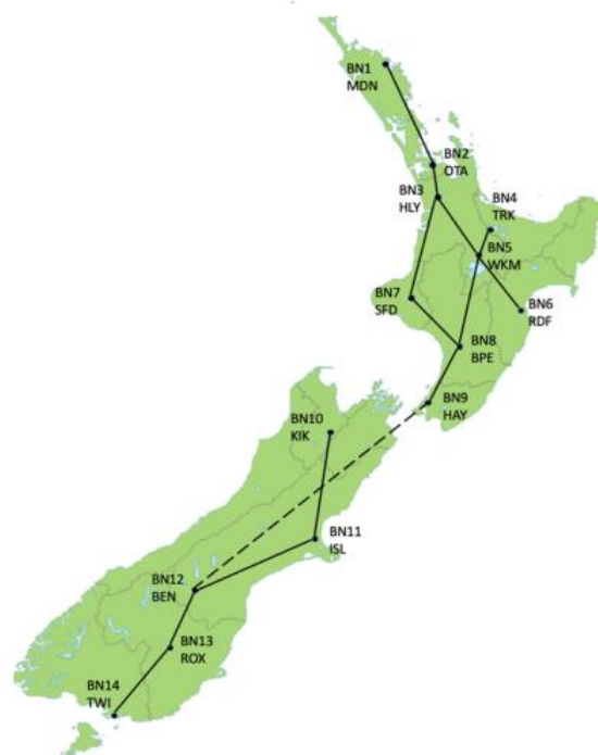
Figure 8 Simplified transmission grid with 14 backbone nodes
