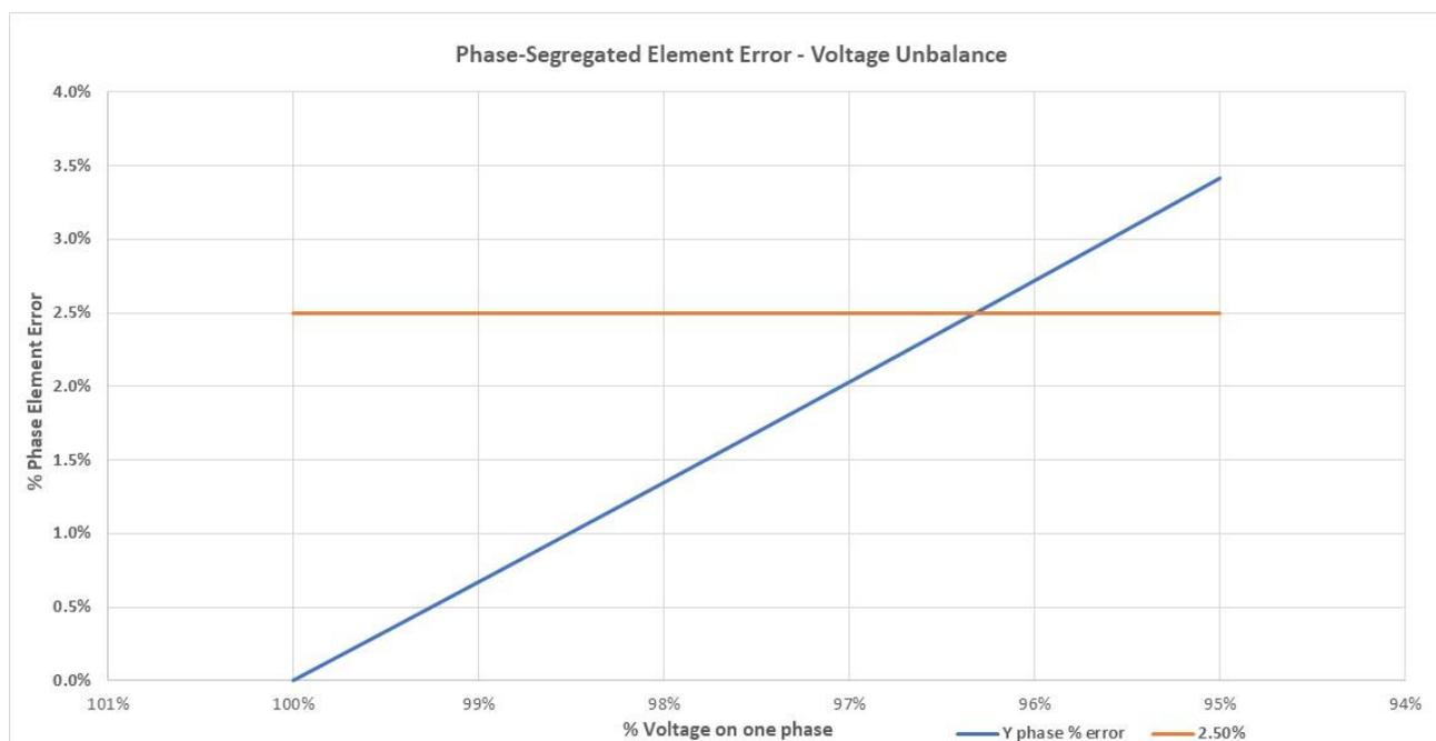
Figure 3: Phase segregated element error with low voltage on one phase
