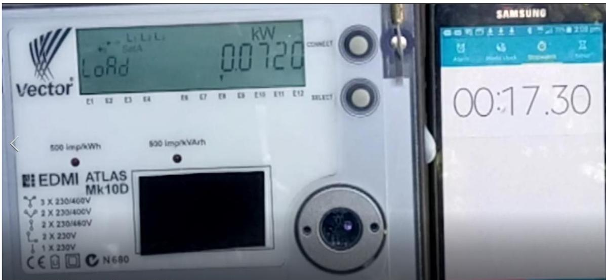
7) At 17 seconds the meter shows an instantaneous kW reading of 0.072 kW (72 W). This is as expected (it is a purely reactive load, there are no actual kW).
