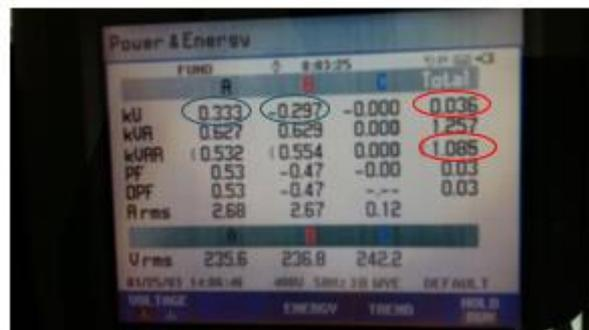
3) We turn all other load off and connect our 5 kVAr load between phases A and B of our installation.
