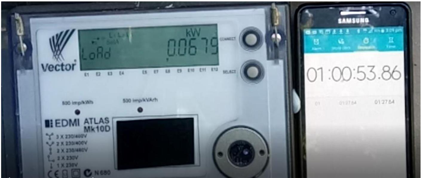
13) The instantaneous meter reading remains essentially unchanged at 0.067 kW.
