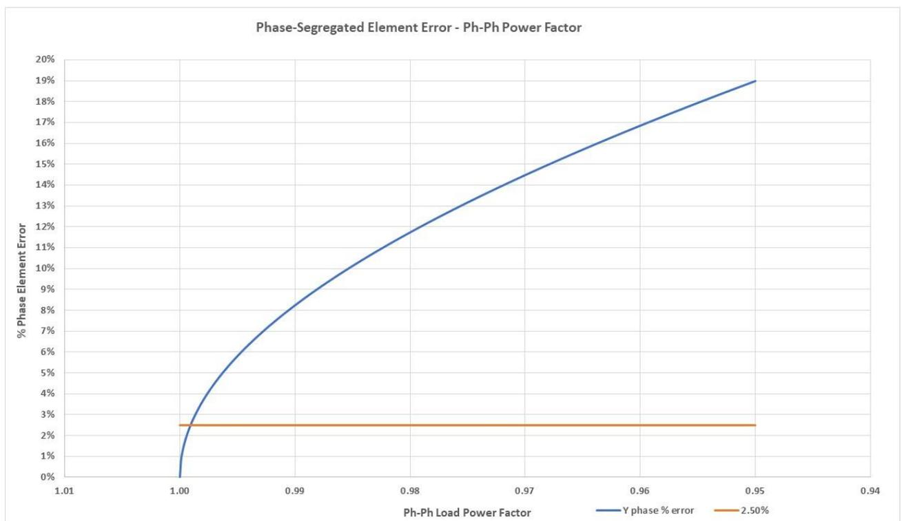
Figure 1: Phase segregated element error with varying load power factor
