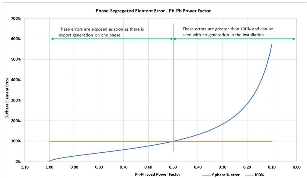
Figure 2: Phase segregated element error at low power factors
