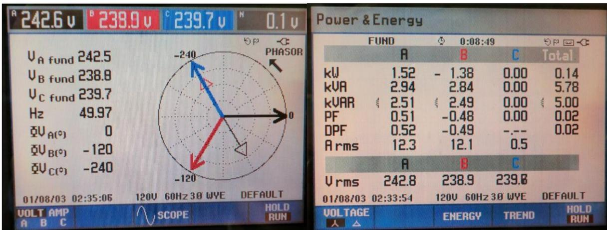
4) As expected, we see a false measurement of +/- 1.5 kW per phase (= 5 x 0.3 kW), with a total load of 0.14 kW (losses) and 5.00 kVAr.
