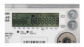
The replacement of these devices with a single electronic meter has led to a reduction of the in-service burden of the installations. However there are a number of the older CTs still in service with higher rated burden.
