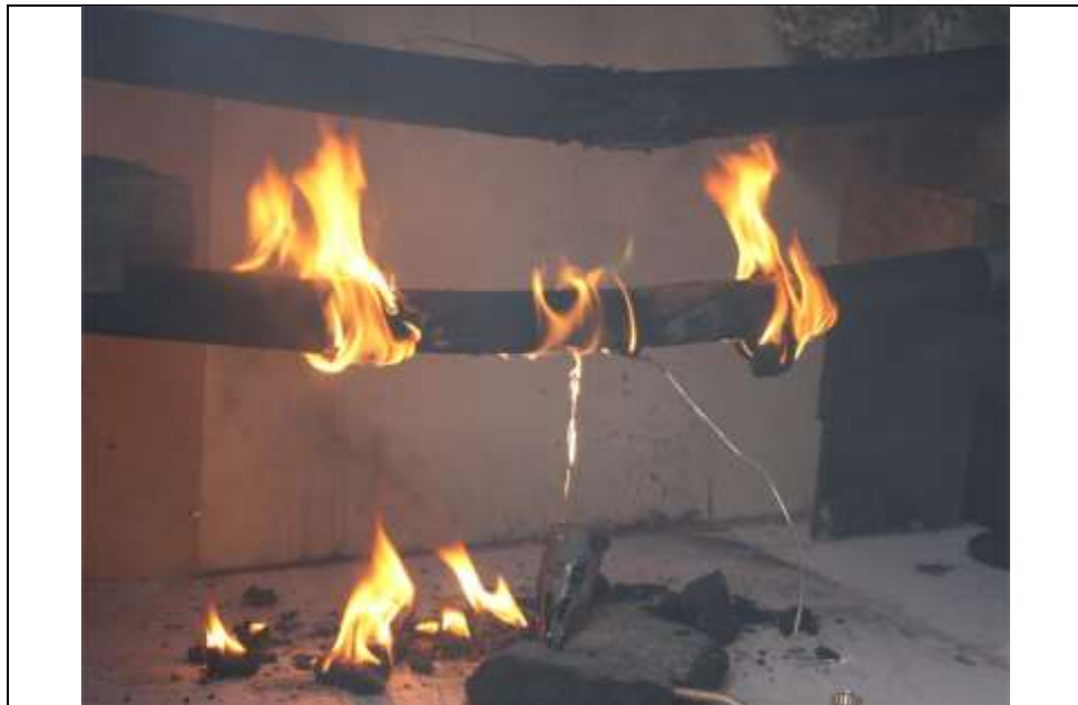
Figure 46 33 kV XLPE cable: flame propagating and PE dropping
