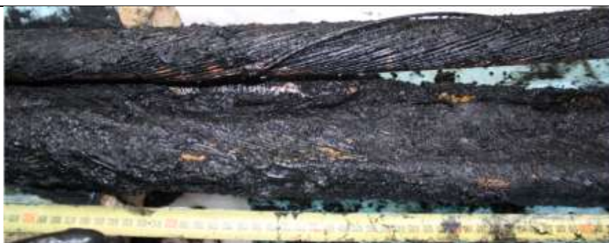
Figure 94 Arc crater: 33 kV XLPE, Sylvia Park No 2, 5DX, 71.8 m
