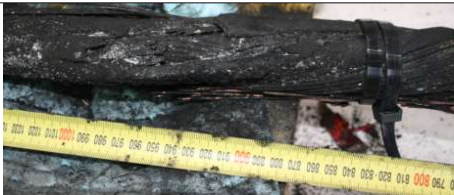
Figure 89 Arc crater: 33 kV XLPE, Mt Wellington N°2, 4EY, 66.9 m
