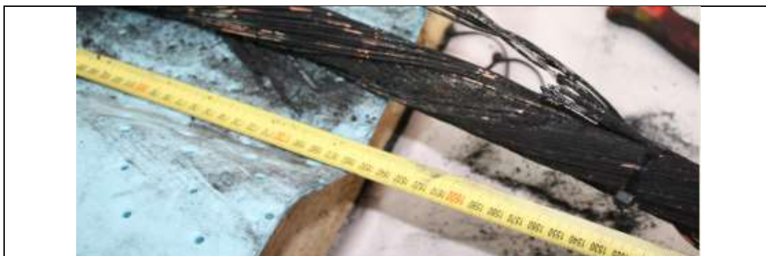
Figure 80 Arc crater: 33 kV XLPE, Remuera 2, 1DY, 72.6 m,
