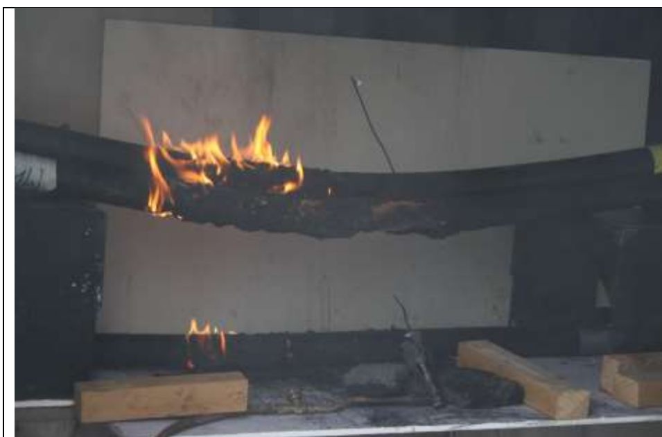
Figure 48 33 kV XLPE trefoil group: flame is sustained
