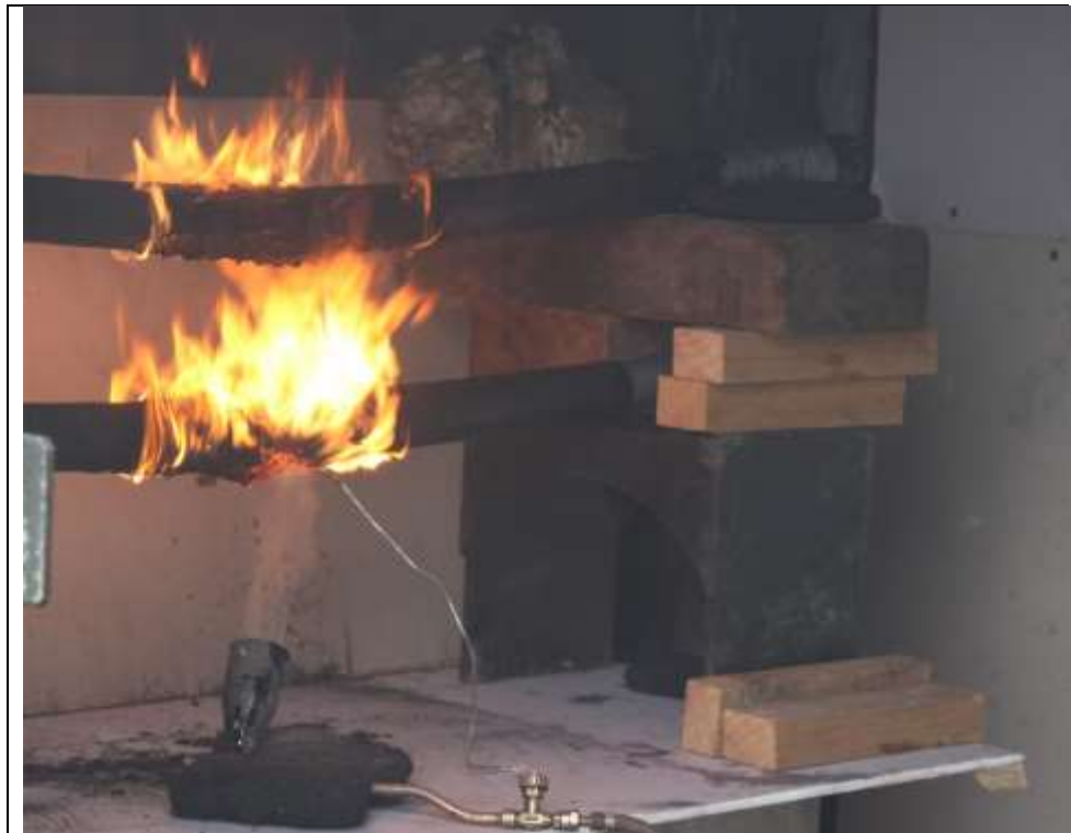
Figure 45 33 kV XLPE cables: ignition of two cables
