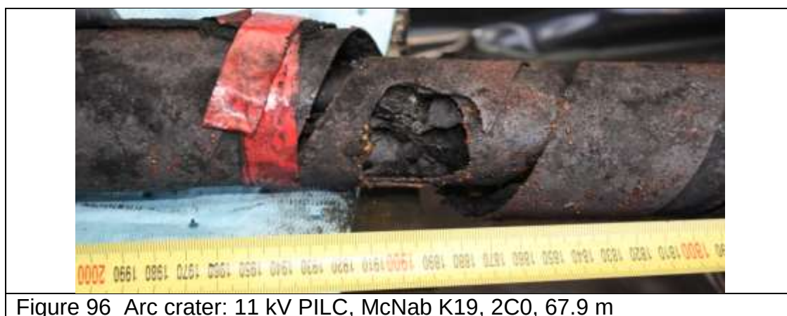
Figure 95 20 th incident: McNab K19 faults: 2C0
