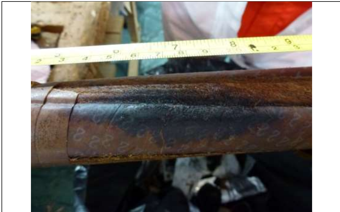
Figure 35 Black feature on the paper insulation of cores No 2 and No 1
