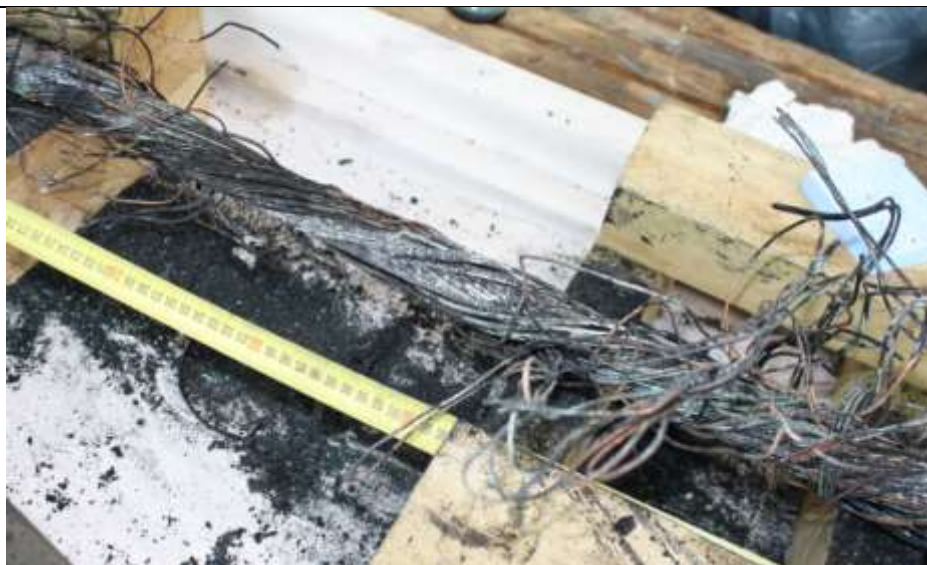
Figure 75 Arc crater: 33 kV XLPE, Newmarket 3, 1B, 73 m, Y Phase
