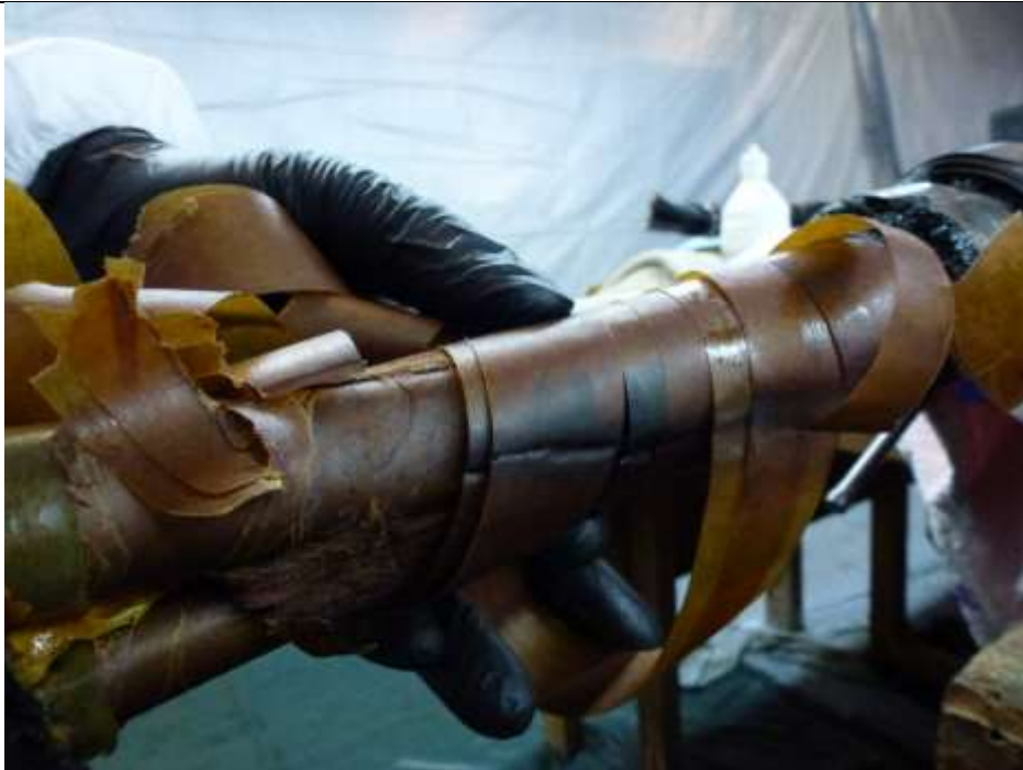
Figure 33 Blackening in belt creases above the core interstices
