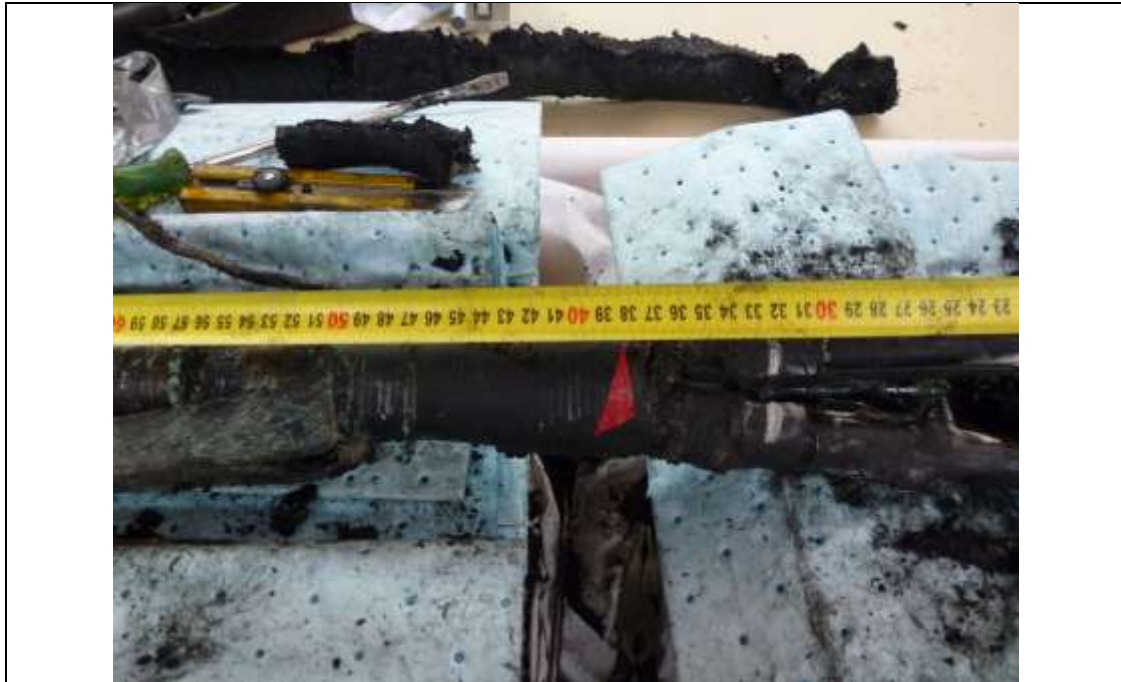
Figure 27 Unfailed joint. Arc centre transferred from failed joint
