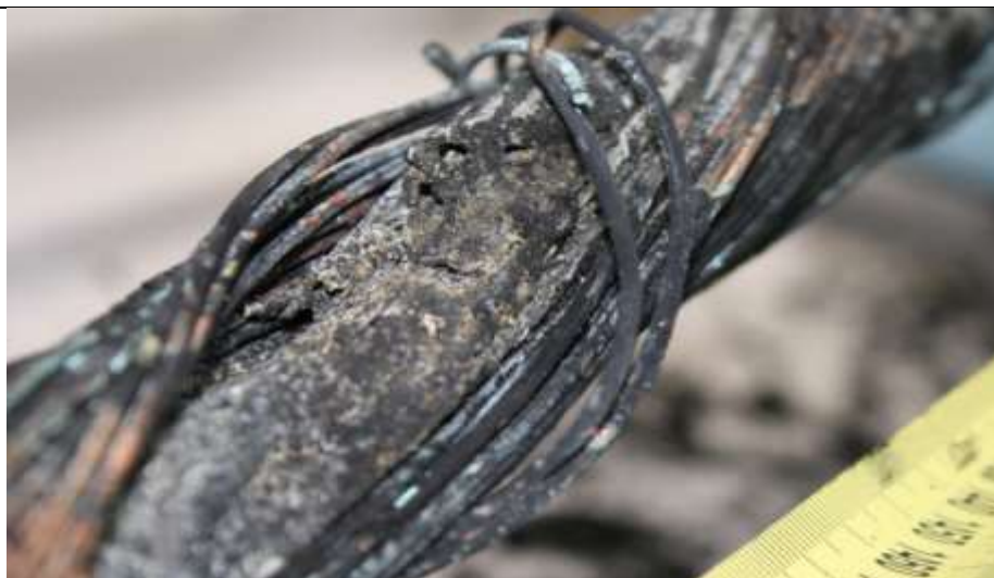
Figure 73 Arc crater: 33 kV XLPE, Remuera 3, 1AZ, 72.5 m
