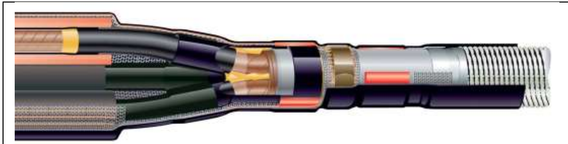
Figure 98 Diagram of an 11 kV three core heatshrink sleeve transition joint PILC to XLPE
