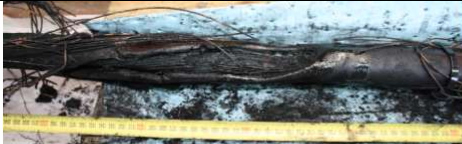
Figure 83 Arc crater: 33 kV XLPE, St John 3, 3FZ, 72.3 m,
