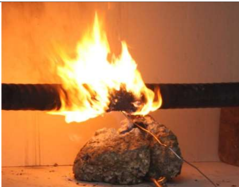
Figure 50 33 kV OF cable: PVC sheath and oil burning
