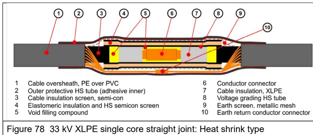
Figure 78 33 kV XLPE single core straight joint: Heat shrink type
