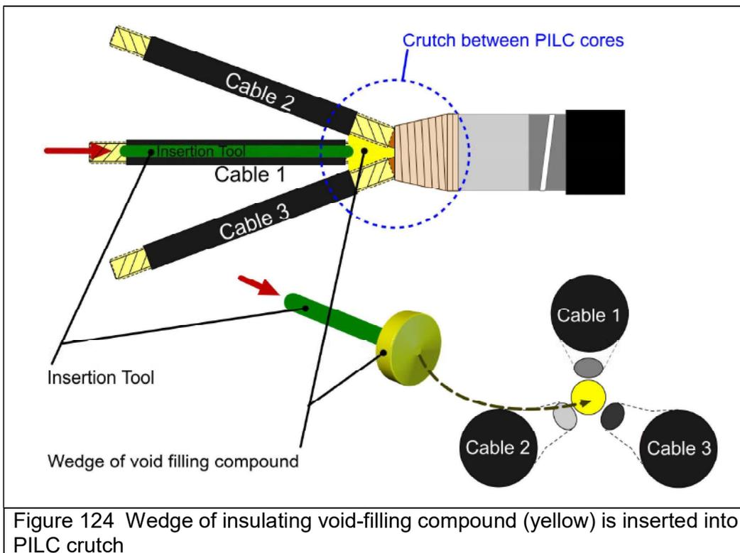
Figure 124 Wedge of insulating void-filling compound (yellow) is inserted into PILC crutch
