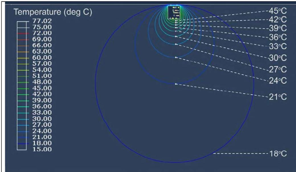
Figure 133 Abaqus-Standard Algorithm model of the cable trench showing ground isothermal lines for winter continuous loading
