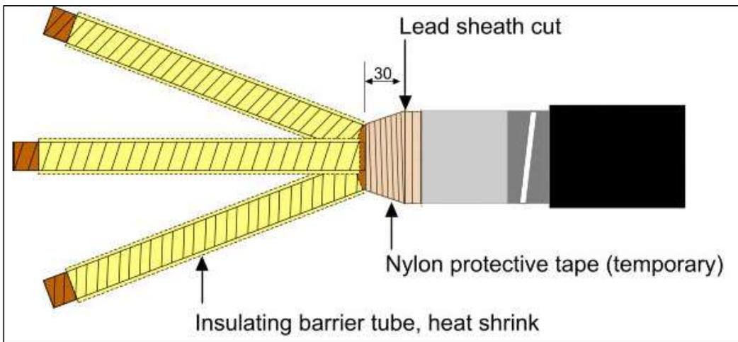
Figure 122 Insulation/barrier tubes are shrunk down over the PILC cores
