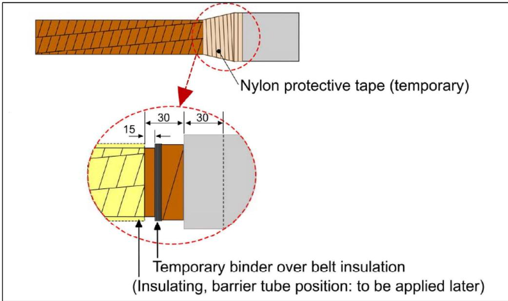
Figure 121 Nylon tapes are applied to protect the core insulation in the crutch
