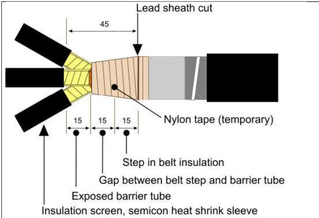
Figure 123 Conductive sleeves (earth screen) are heat shrunk onto the insulation/barrier tubes
