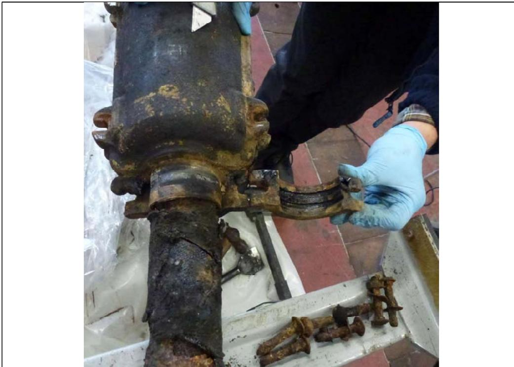
Figure 75 Cable clamp: Cast iron on lead tape packing
