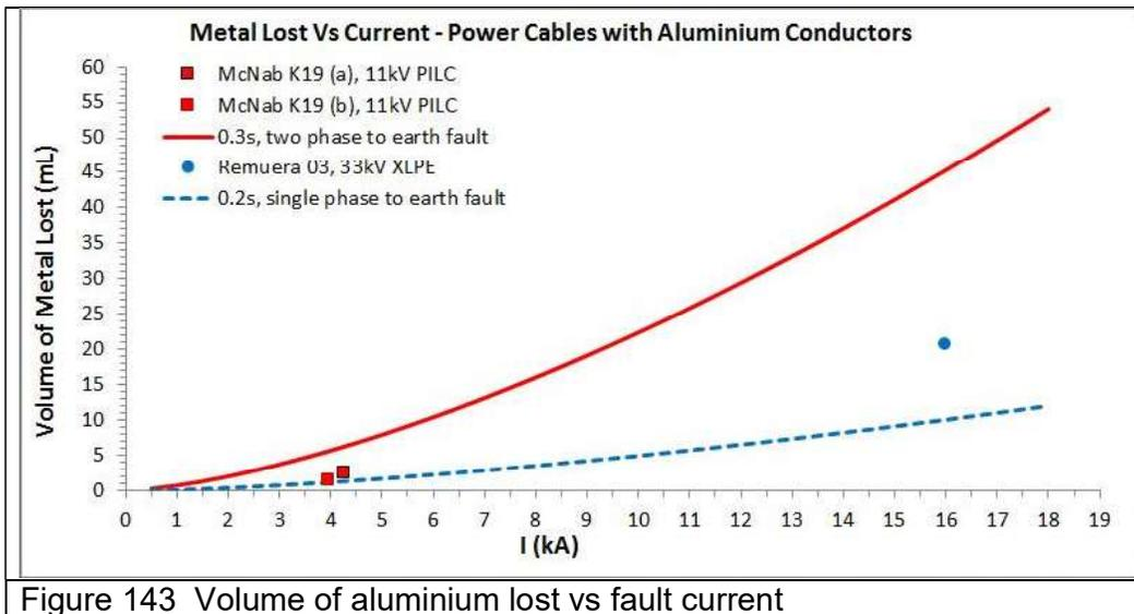
Figure 143 Volume of aluminium lost vs fault current
