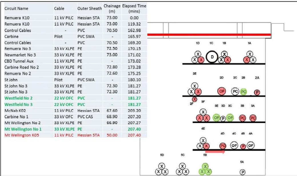
Figure 106 18th incident: 11 kV PILC, Mt Wellington K05 fault: 4D0, 50 m
