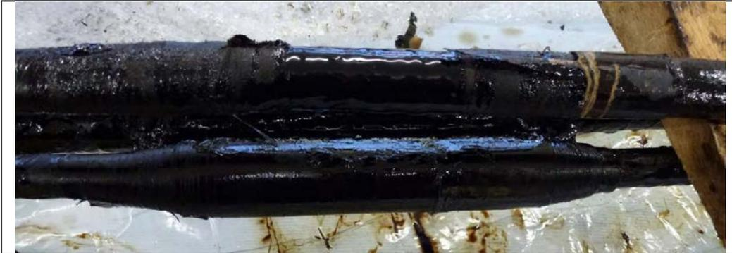
Figure 70 Connector insulation: Pre-shaped paper rolls
