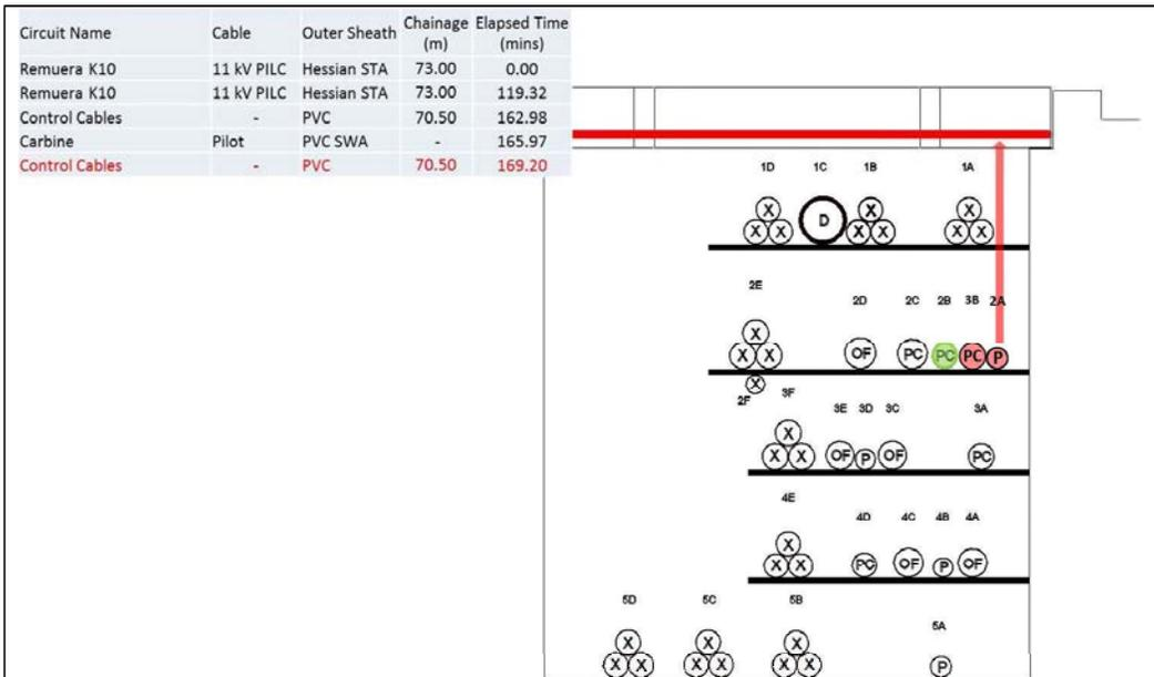
Figure 86 5th incident: Control cable signal across the cable bridge, 70.5 m
