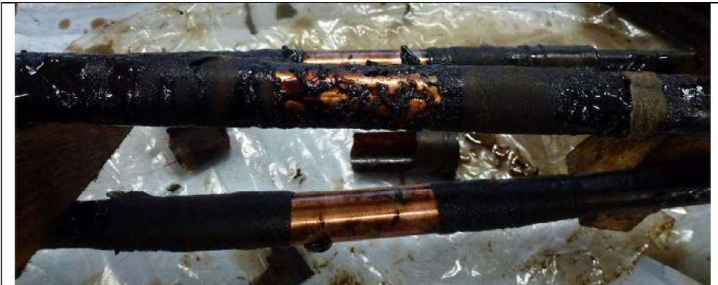
Figure 69 Connector infill insulation: Impregnated cotton tape
