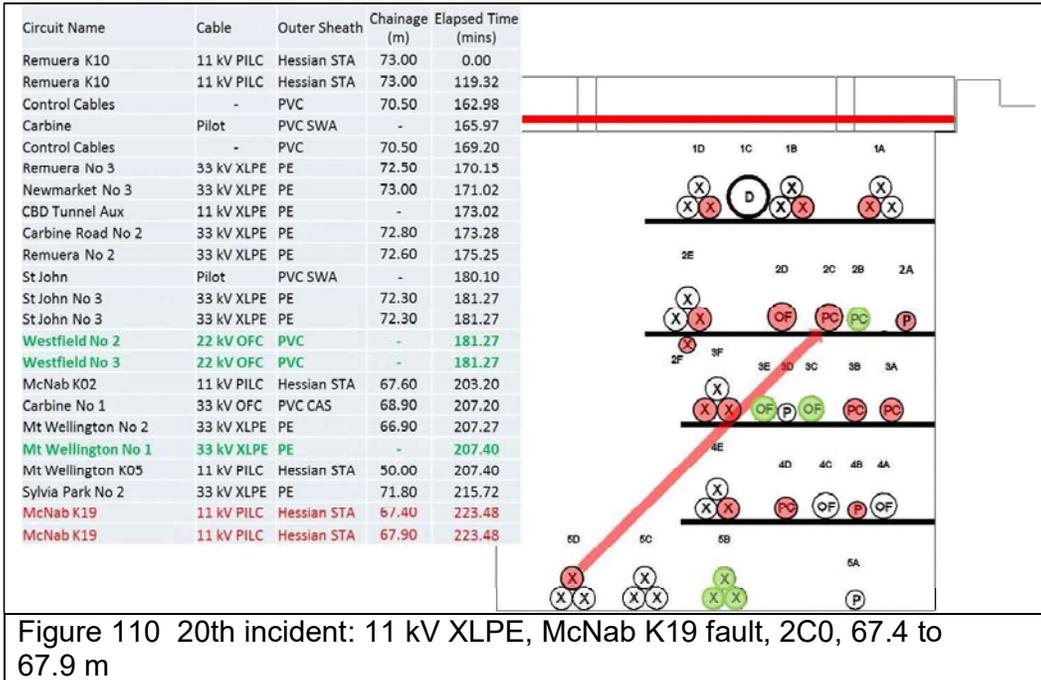
Figure 110 20th incident: 11 kV XLPE, McNab K19 fault, 2C0, 67.4 to 67.9 m
