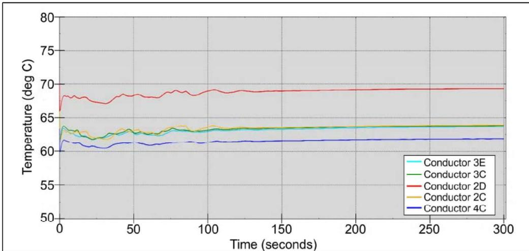
Figure 130 Temperature rise with time: continuous steady state loading at summer peak currents. Abaqus-CFD convection method
