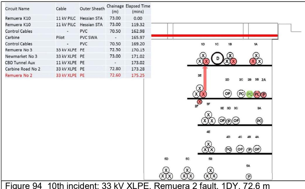
Figure 94 10th incident: 33 kV XLPE, Remuera 2 fault, 1DY, 72.6 m
