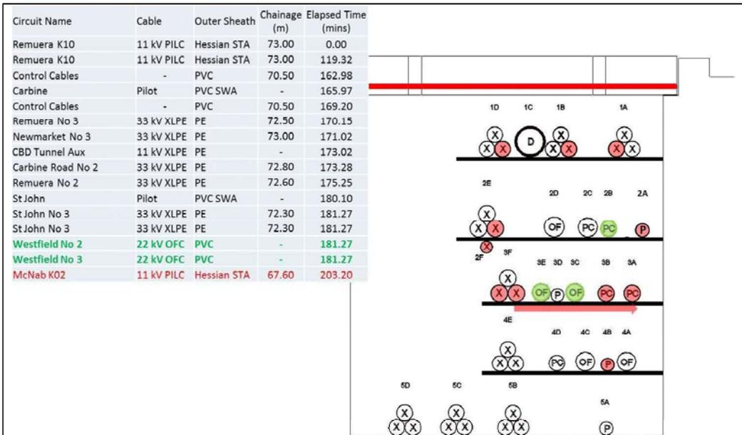
Figure 100 14th incident: 11 kV PILC, McNab K02 fault, 3A0, 67.6 m
