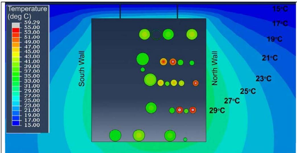
Figure 136 Winter 2 h peak 24 h cyclic rating (Abaqus-Standard): Cable and ground temperatures
