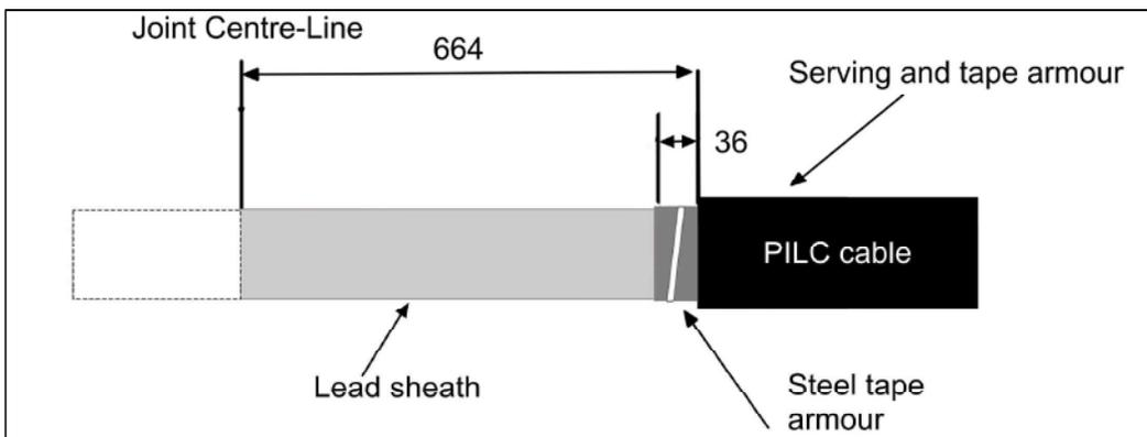
Figure 118 Serving and armour are stripped off the PILC lead sheath
