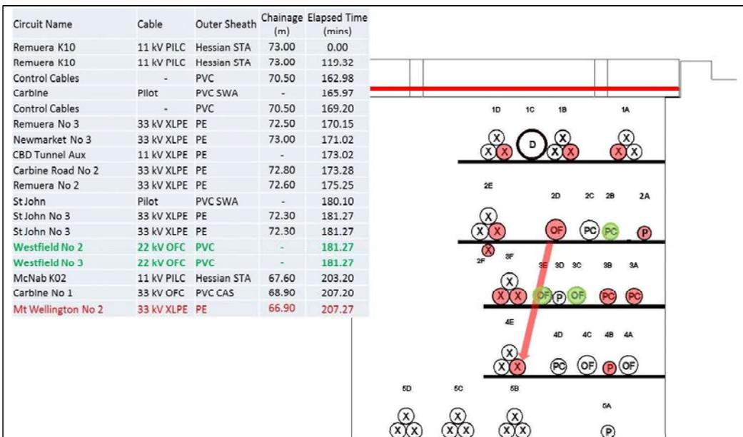
Figure 103 16th incident: 33 kV XLPE, Mt Wellington No2 fault, 4EY, 66.9 m
