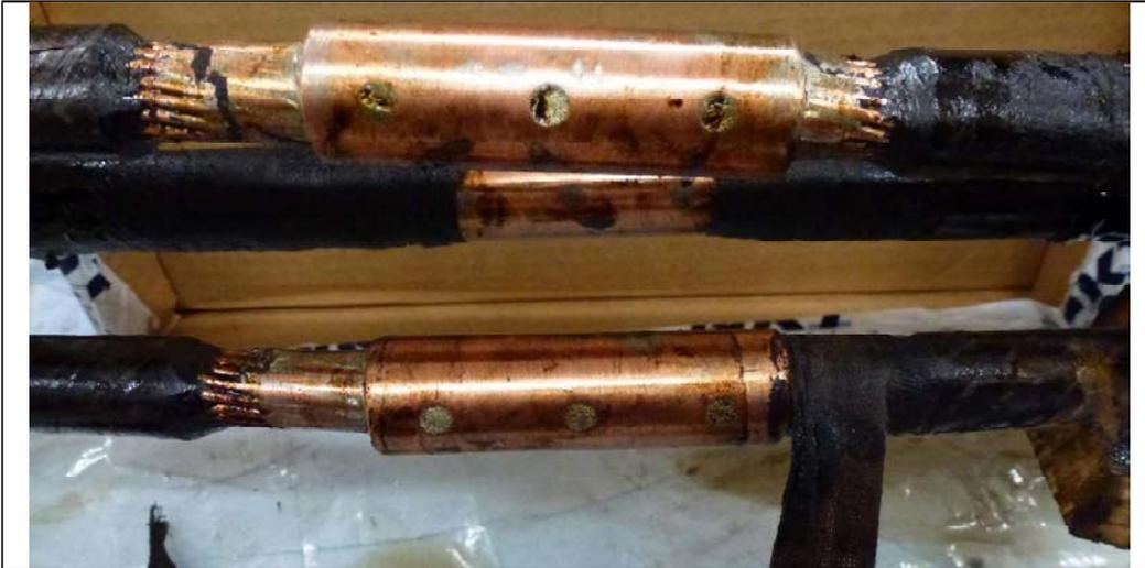
Figure 68 Conductor connectors: Copper ferrule sweated with tin-lead alloy
