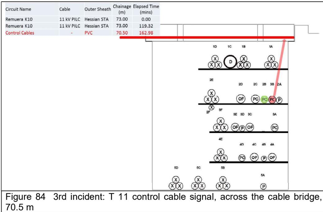
Figure 84 3rd incident: T 11 control cable signal, across the cable bridge, 70.5 m
