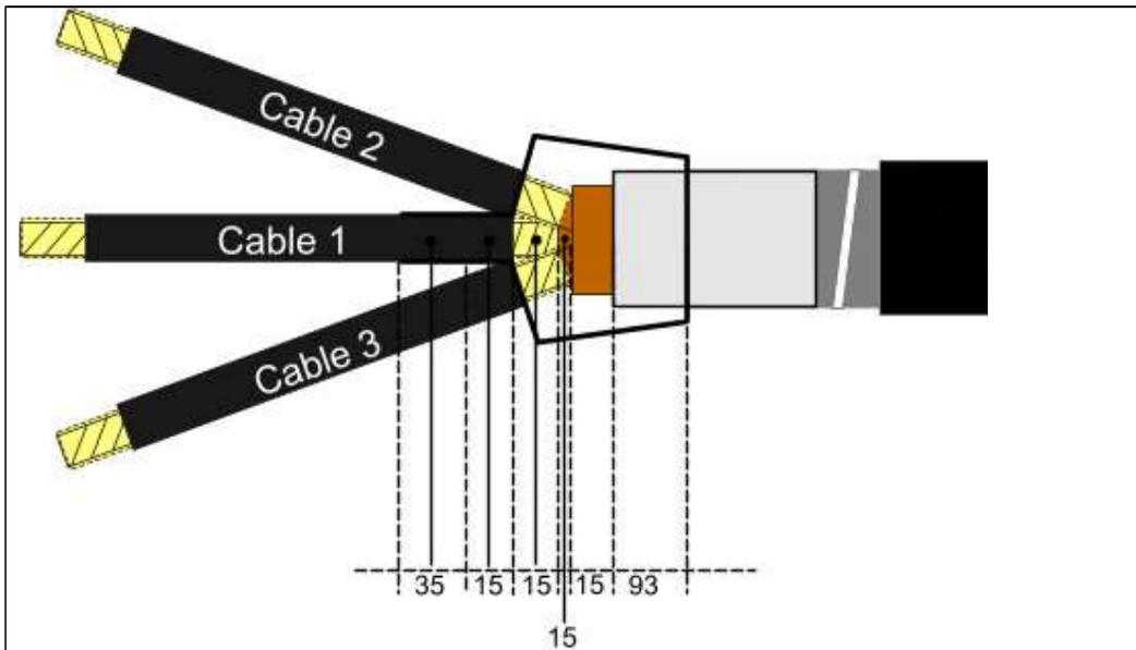
Figure 128 Dimensions of components associated with the break-out glove
