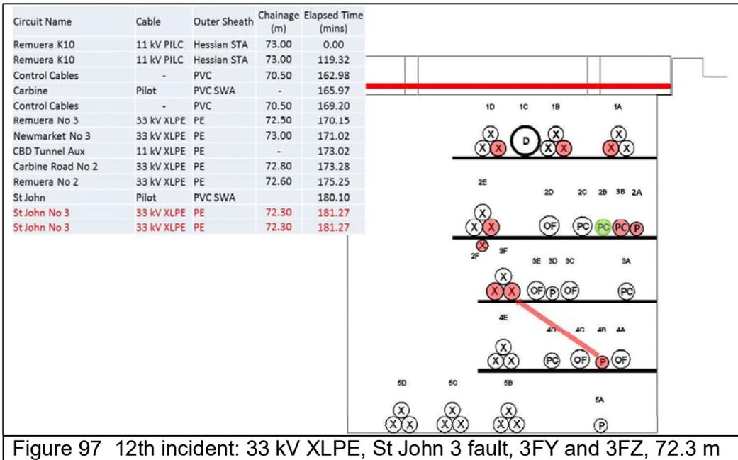
Figure 97 12th incident: 33 kV XLPE, St John 3 fault, 3FY and 3FZ, 72.3 m
