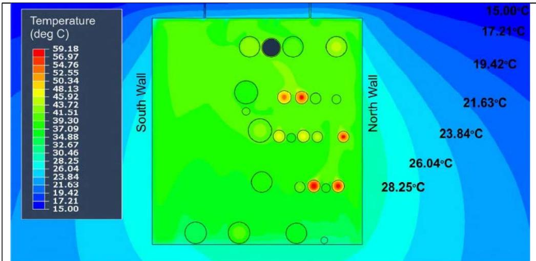
Figure 138 Winter 2 h peak 24 h cyclic rating (Abaqus CFD): Conductor, cable, air and ground temperatures
