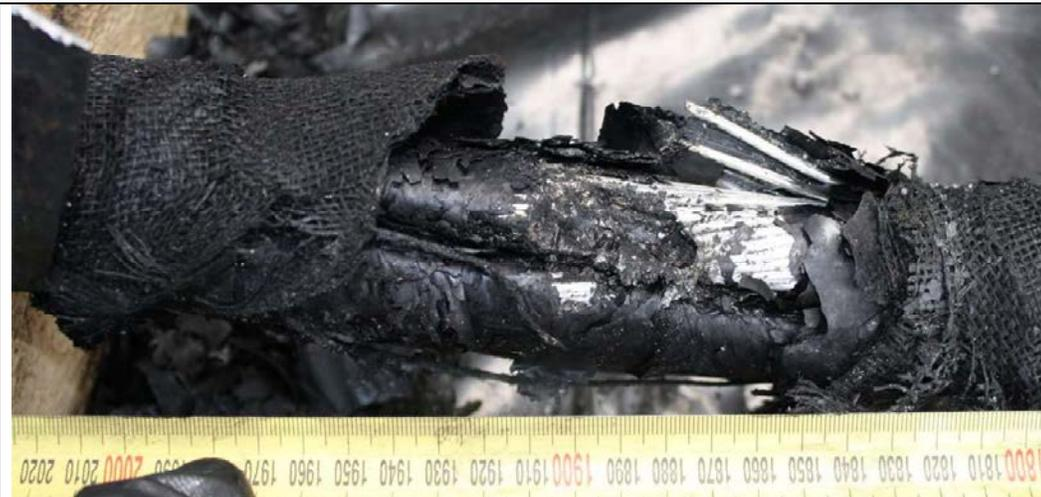
Figure 112 Arc crater in conductor: 11 kV PILC, McNab K19, 2C0, 67.4 to 67.9 m
