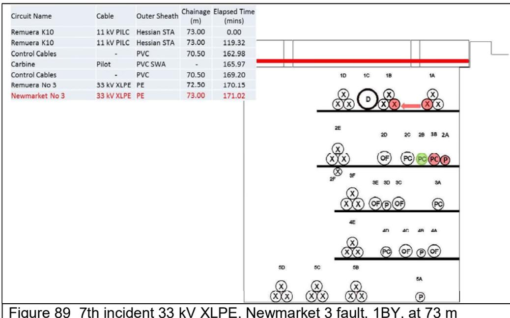
Figure 89 7th incident 33 kV XLPE, Newmarket 3 fault, 1BY, at 73 m
