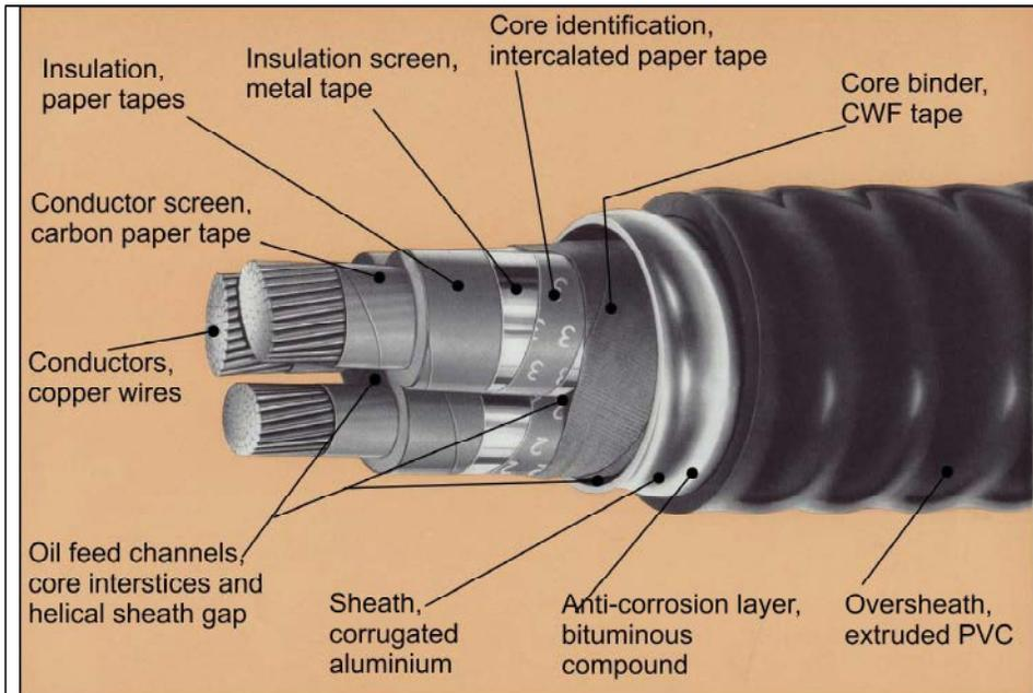
Figure 76 33 kV oil-filled three core cable
