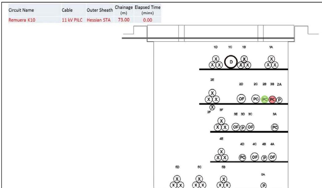
Figure 81 1st incident: 11 kV PILC, Remuera K10 fault, 3B0, 73 m
