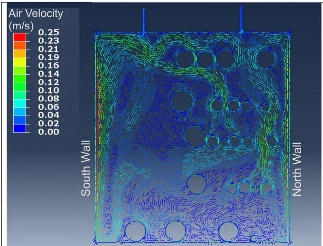
Figure 139 Winter 2 h peak 24 h cyclic rating (Abaqus: CFD): Velocity vector plot of air convection
