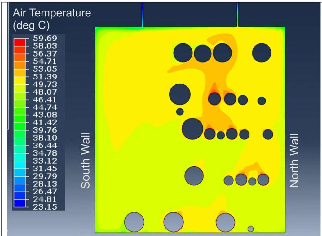
Figure 132 Air temperature contour plot: continuous steady state loading at the summer peak current values. Abaqus-CFD convection method
