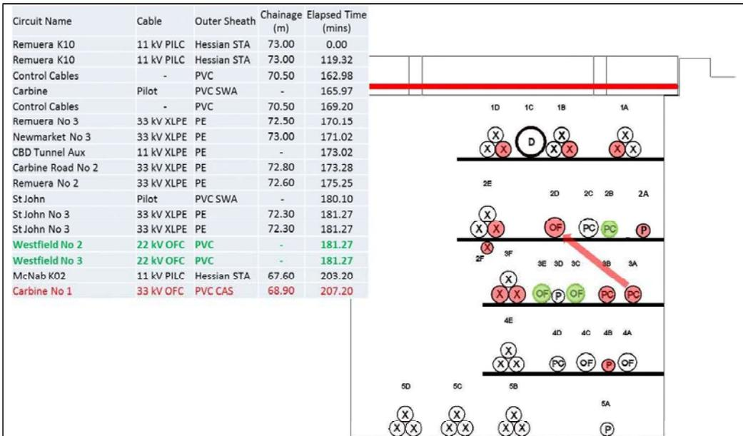
Figure 101 15th incident: 33 kV OF, Carbine No1 fault, 2D0, 68.9 m
