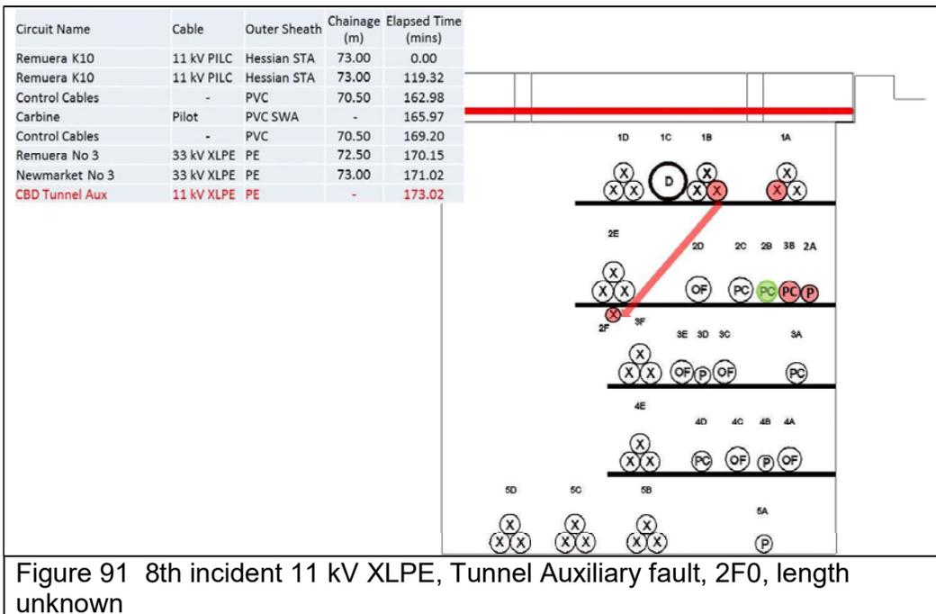
Figure 91 8th incident 11 kV XLPE, Tunnel Auxiliary fault, 2F0, length unknown
