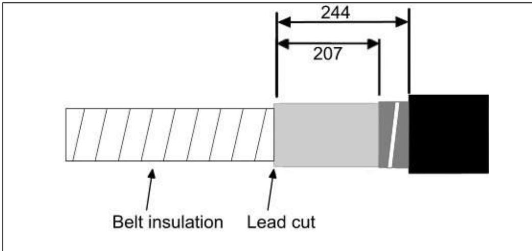
Figure 119 Lead sheath is removed from PILC cable to the lead cut position
