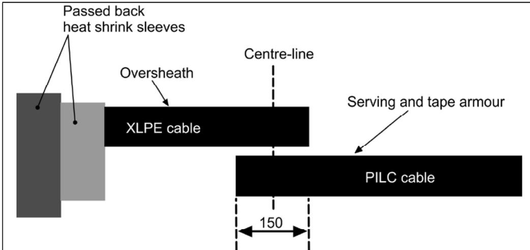
Figure 117 Outer protective heat shrink sleeves are passed-back
