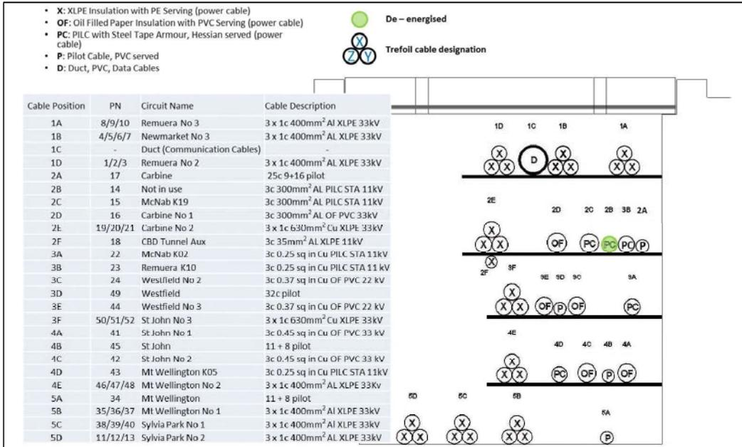
Figure 80 Layout of circuits in the trench
