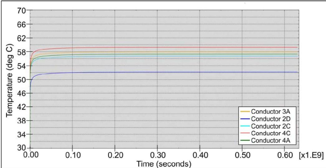
Figure 137 Winter 2 h peak 24 hour cyclic rating (Abaqus-Standard): Cable temperatures
