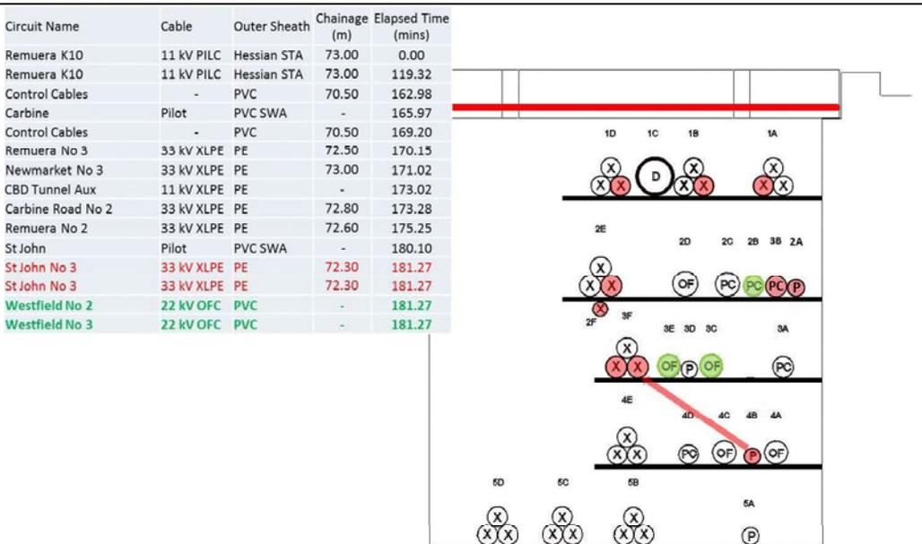
Figure 99 13th incident: 22 kV OF, Westfield 2 and 3 are opened unfailed, 3C0 and 3E0
