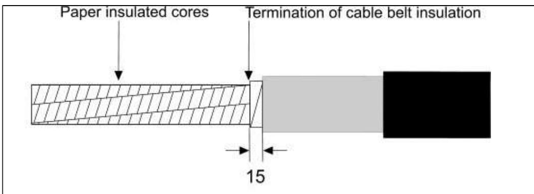
Figure 120 PILC belt tapes are torn off to form the belt insulation step
