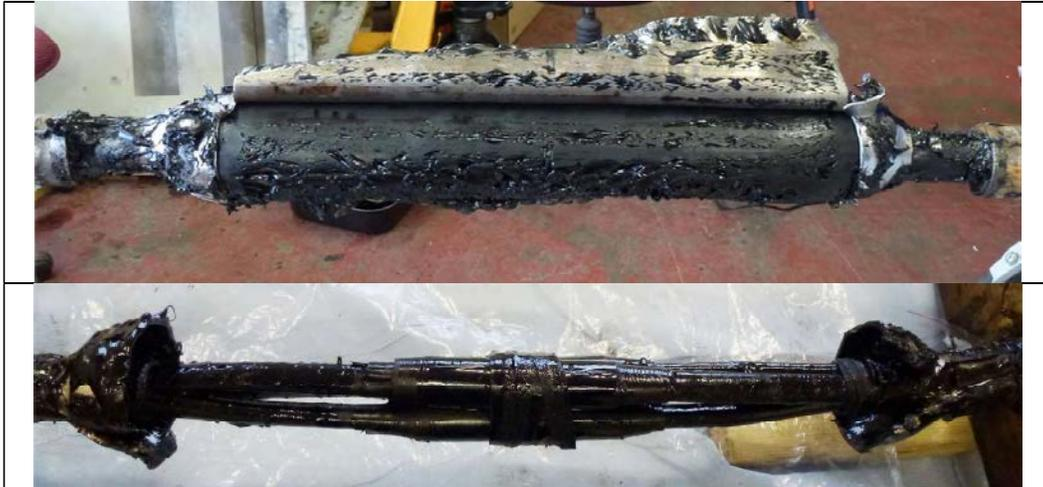
Figure 72 Bitumen filled lead sleeve and encapsulated core insulation
