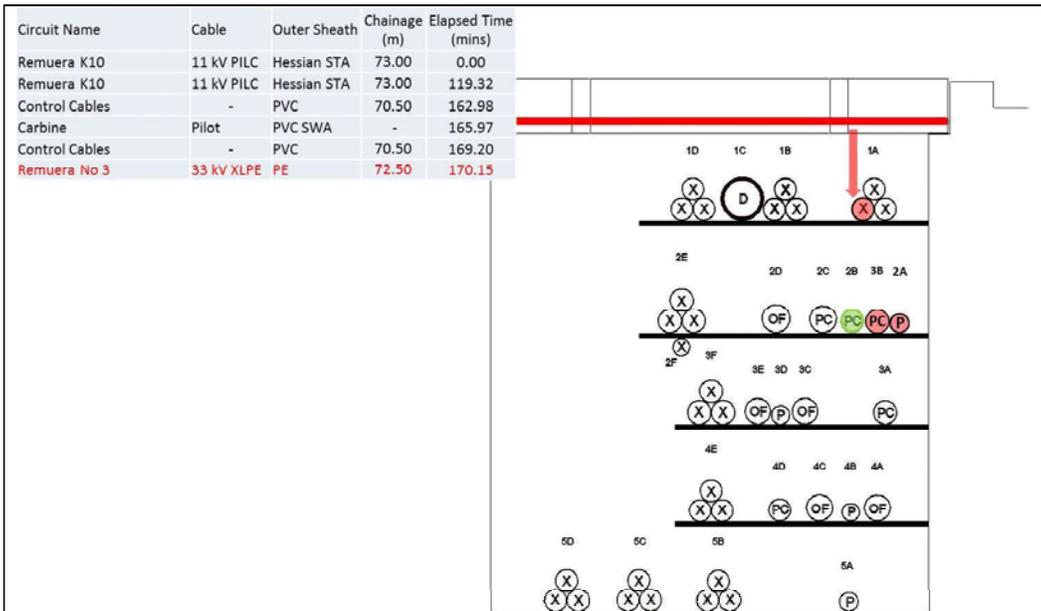
Figure 87 6th incident: 33 kV XLPE, Remuera 3 fault, 1AZ, 72.5 m
