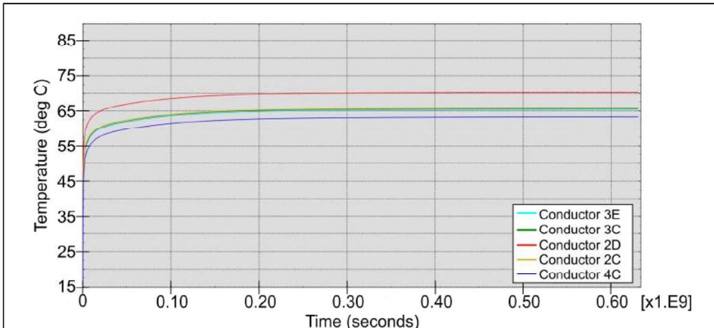
Figure 129 Temperature rise with time; continuous steady state loading at summer peak currents. Abaqus-Standard using convection algorithm equation:
