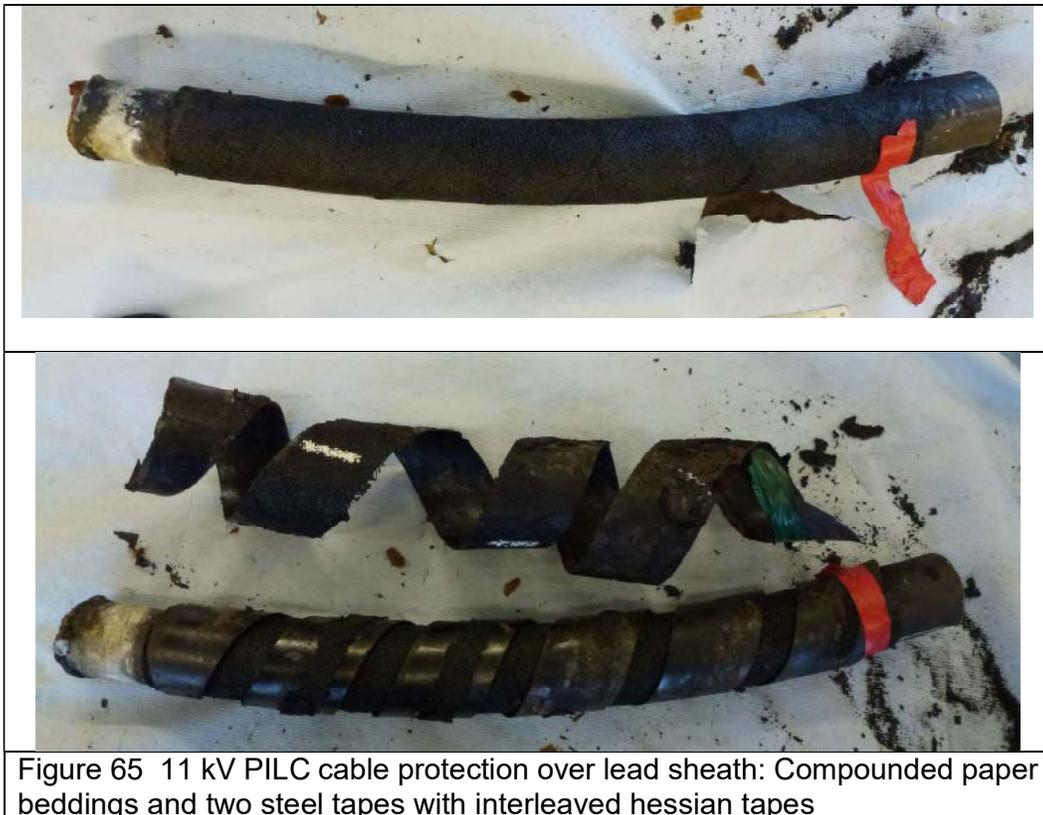
Figure 65 11 kV PILC cable protection over lead sheath: Compounded paper beddings and two steel tapes with interleaved hessian tapes
