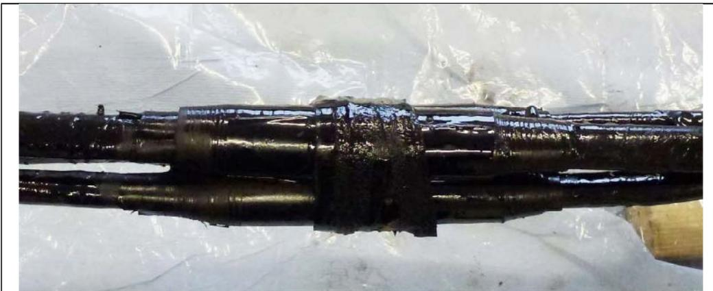
Figure 71 Binder and spacer: Cotton fabric tape over common paper roll
