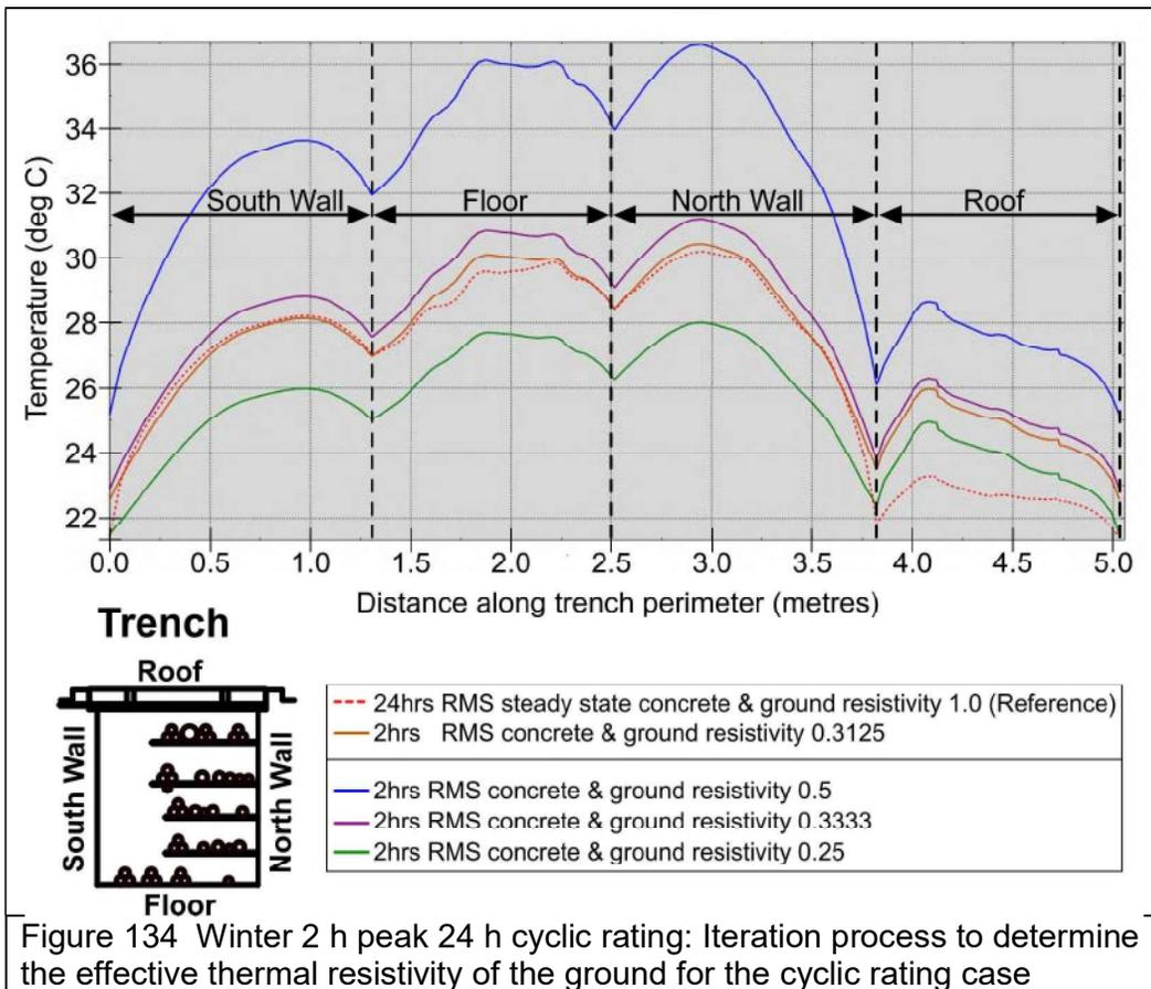
Having achieved the same wall and floor temperatures with a ground and wall thermal resistivity of 0.3125 Km/W, the conductor temperatures under cyclic loading were abstracted. Table 12 compares the conductor temperatures under winter cyclic loading calculated using the Abaqus-CFD co-simulation with the Abaqus-Algorithm simulation methods.
