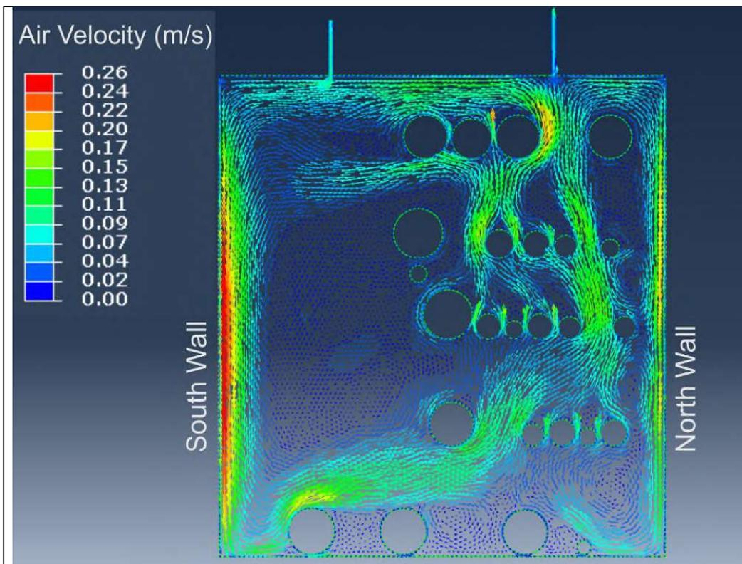
Figure 131 Velocity vector plot of air convection: continuous steady state loading at the summer peak current. Abaqus-CFD convection method
