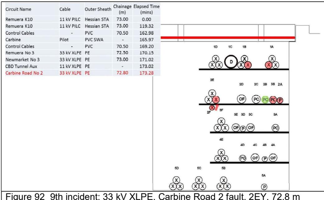
Figure 92 9th incident: 33 kV XLPE, Carbine Road 2 fault, 2EY, 72.8 m
