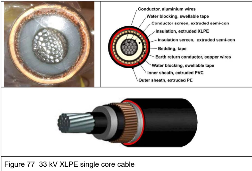
In the cable trench three phase circuits were formed by laying three single core cables in trefoil-touching formations. At 33 kV it is generally preferred by utilities to select single core rather than three core cables as the XLPE insulation thickness is sufficient to make installation of a three core cable less flexible and the three core construction to make the joint larger and jointing more complex.
