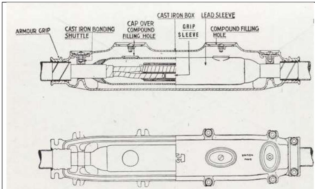
Figure 66 11 kV PILC three core straight joint: Cast iron shell type
