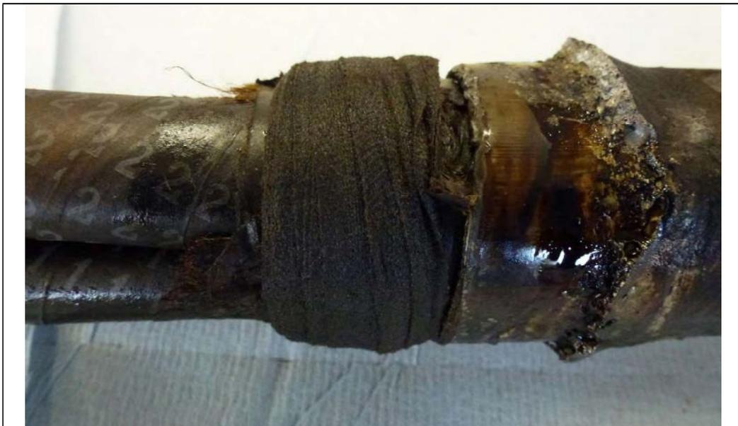
Figure 67 Belt insulation binder at lead sheath cut: Impregnated cotton tape
