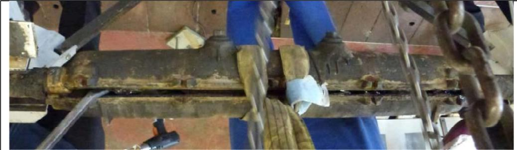
Figure 74 Joint shell halves: Cast iron filled with bituminous compound
