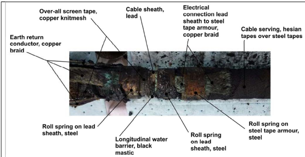
Figure 116 Electrical connections to PILC lead sheath and armour tapes
