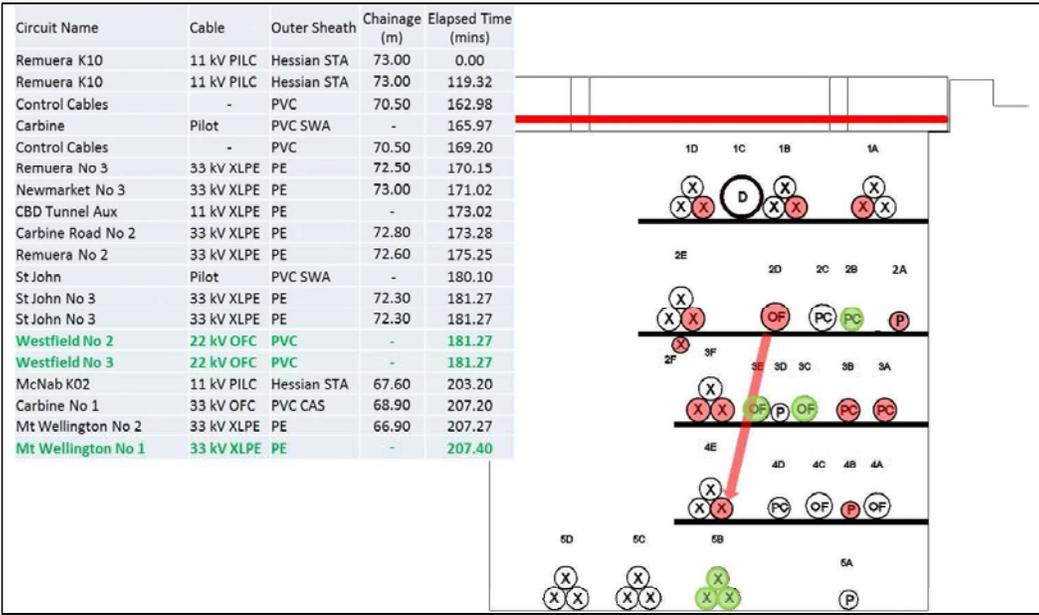
Figure 105 17th incident: 33 kV XLPE Mt Wellington No1 tripped, 5B
