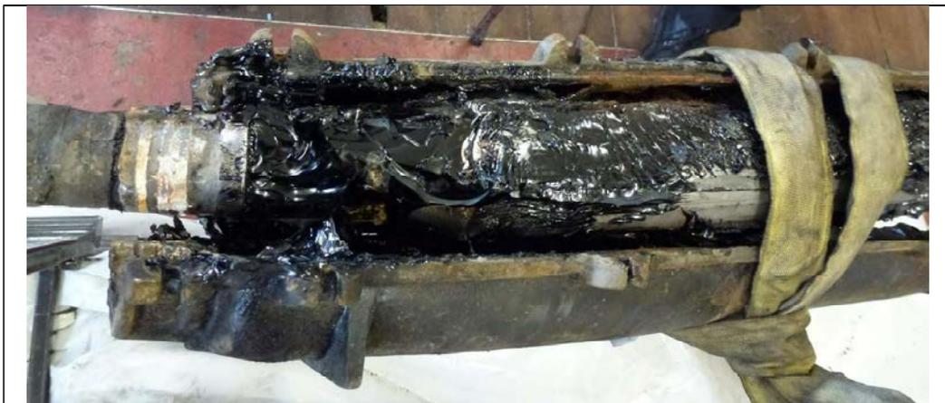
Figure 73 Inner watertight barrier: Wiped lead sleeve encapsulated within bituminous anti-corrosion protection
