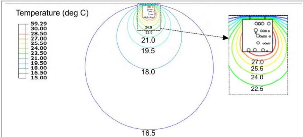
Figure 135 Winter 2 hour peak 24 hour cyclic rating (Abaqus-Standard): Ground isotherms
