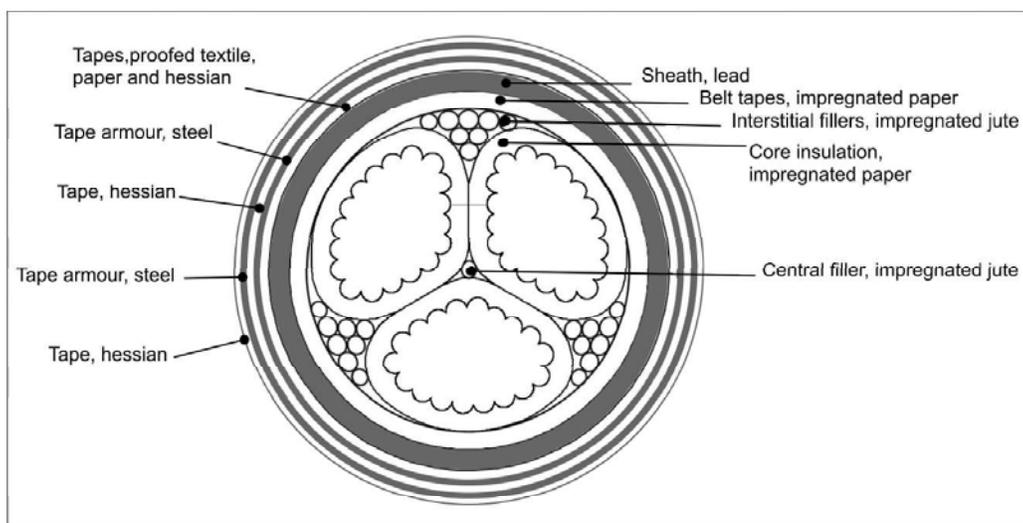
Figure 64 11 kV PILC three core cable cross-sections
