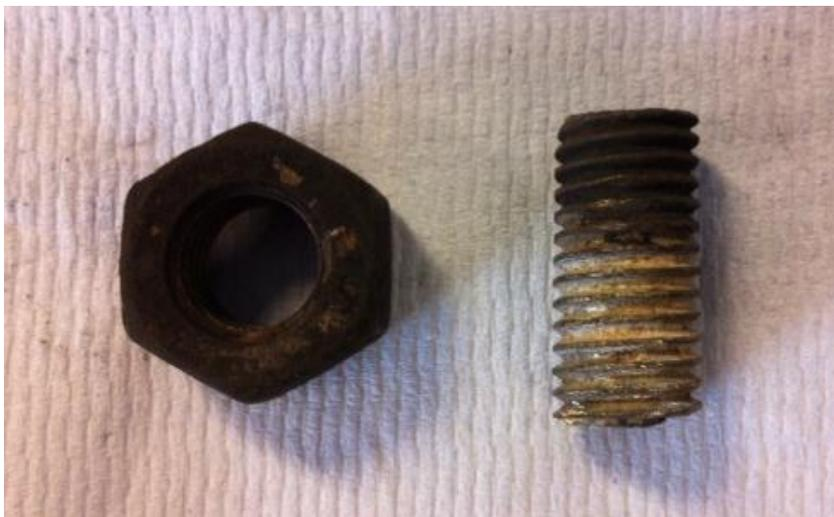
Figure 49: PN67 bottom stud and nut 69m
