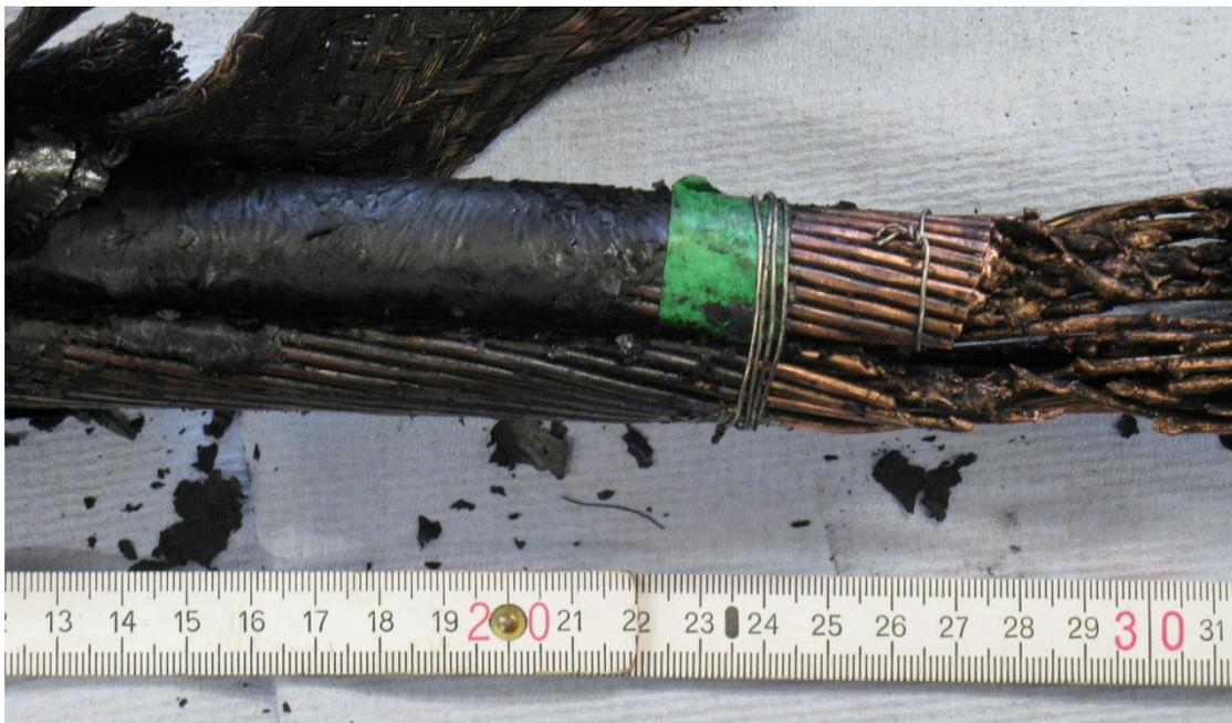
**Figure 9: Closer view of core papers on faulted transition joint**
