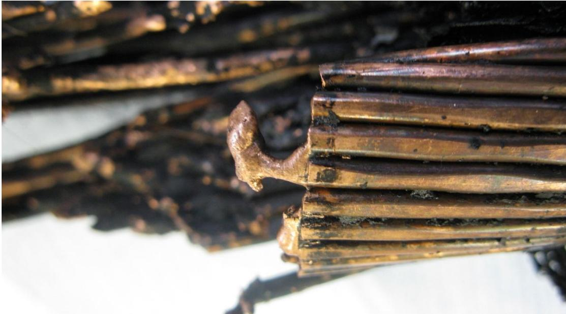
**Figure 4: Arc eroded end of green labelled core on cable side of fault**
