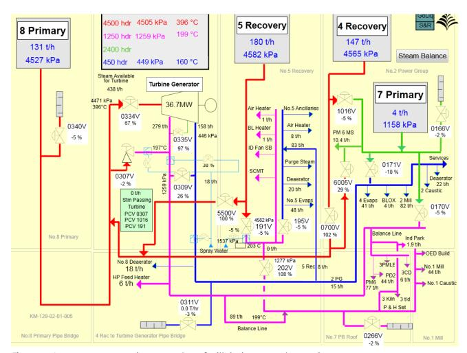
Figure 1. Steam system overview; snapshot of mill during normal operation.
