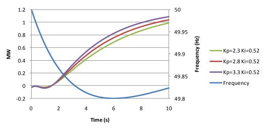
Figure 9: Machine B with Varying Proportional Gain
