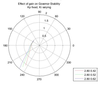
Figure 12: Nyquist plot showing the effect of Integral gain on machine B
