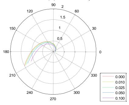
Figure 5: Nyquist plot showing the effect of dead band on machine A
