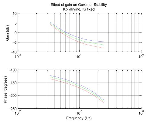
Figure 20: Bode plot showing the effect of Proportional gain on machine B
