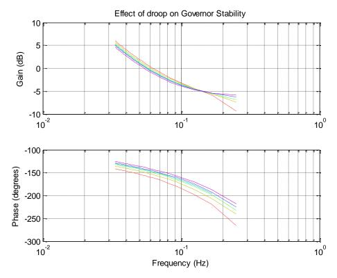
Figure 18: Bode plot showing the effect of droop on machine B
