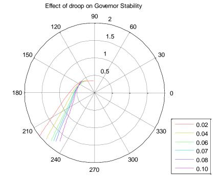
Figure 8: Nyquist plot showing the effect of droop on machine B
