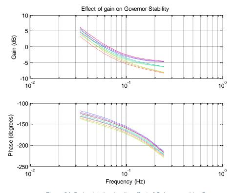
Figure 24: Bode plot showing the effect of Gain on machine B
