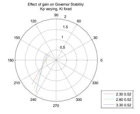
Figure 10: Nyquist plot showing the effect of Proportional gain on machine B
