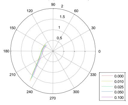
Figure 6: Nyquist plot showing the effect of dead band on machine B
