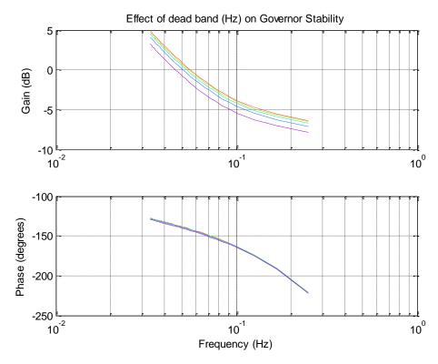
Figure 16: Bode plot showing the effect of dead band on machine B
