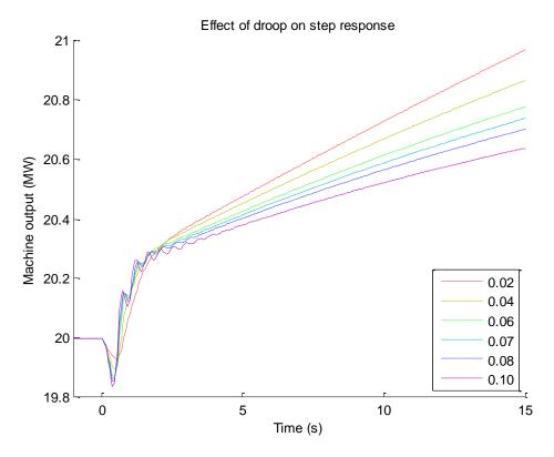
Figure 7: Step response test on machine B
