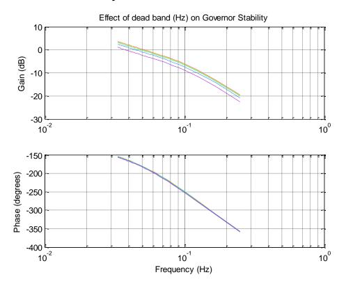
Figure 14: Bode plot showing the effect of dead band on machine A
