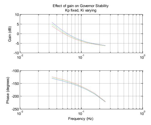
Figure 22: Bode plot showing the effect of Integral gain on machine B
