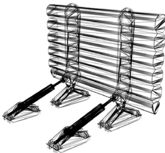
Figure 2.5: Aquamarine's Oyster Surge Device Design
