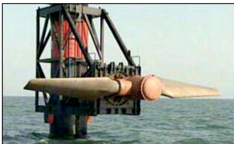
Figure 2.11: The 300 kW SeaFlow Prototype at Lynmouth, Devon
