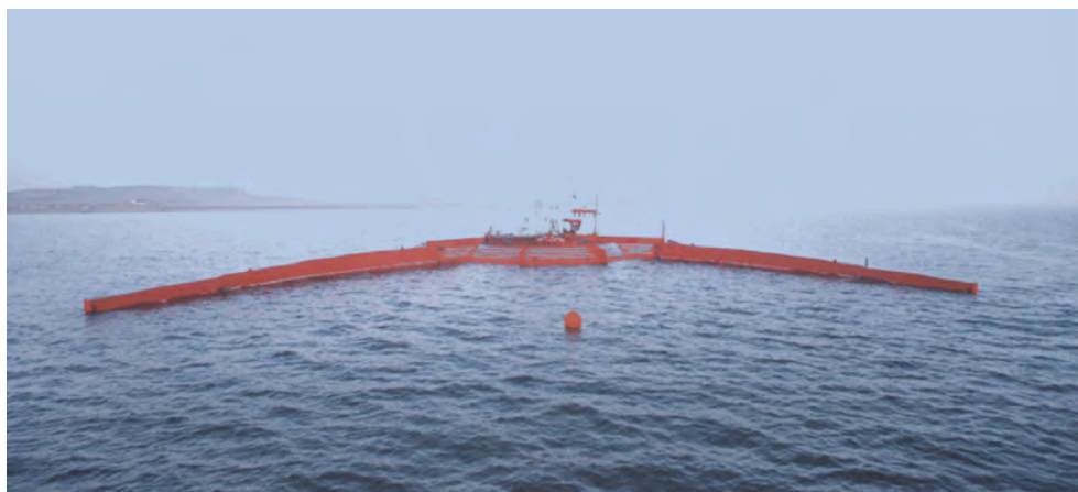
Figure 2.4: ~1/4-scale Wave Dragon in Nissum Bredning, Denmark
